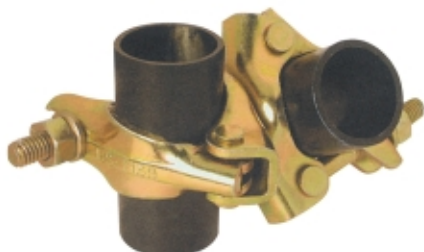
JK-014 SWIVEL COUPLER For Pipe OD 48.3 mm (EN-74 / BS-1139)
